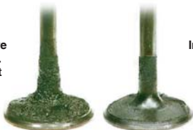
Intake Valve before P.i. Treatment
